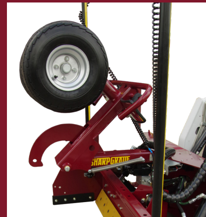
Retracting wheels for confined space / transport
