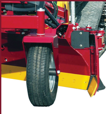
Hydraulic wings control material in both directions
