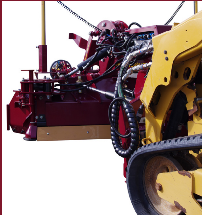
Rear blade to precision grade in reverse
