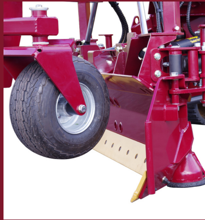
Hydraulic wings control material in both directions
