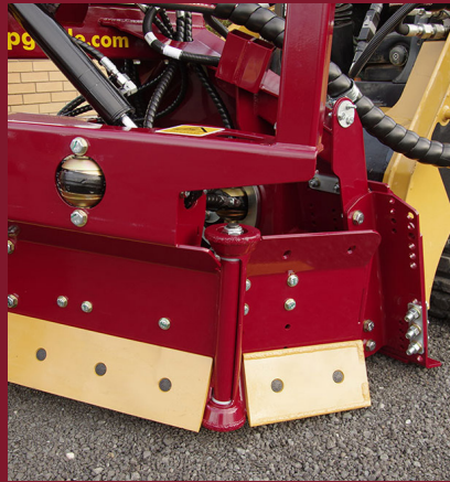
Hydraulic wings control material in both directions
