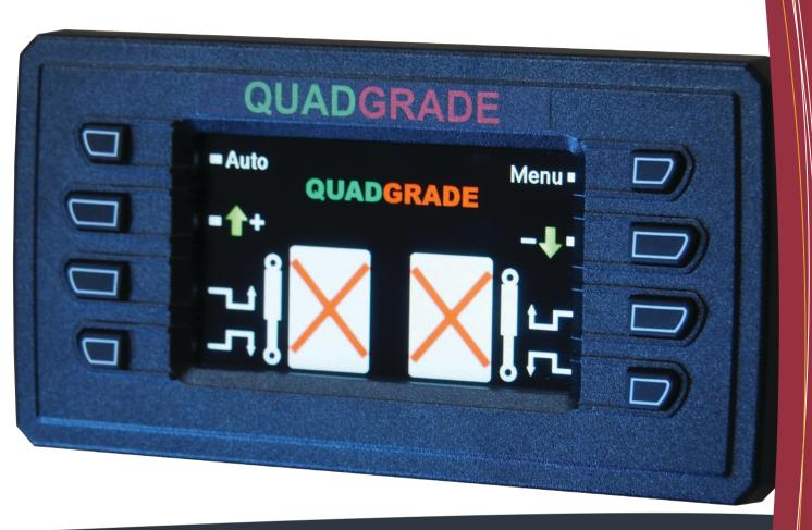
Compact, waterproof 2D control system for box blade levellers
